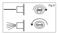
The spray is adjustable from a pencil jet spray to fan spray by tuning the nozzle shown (Fig 8).
